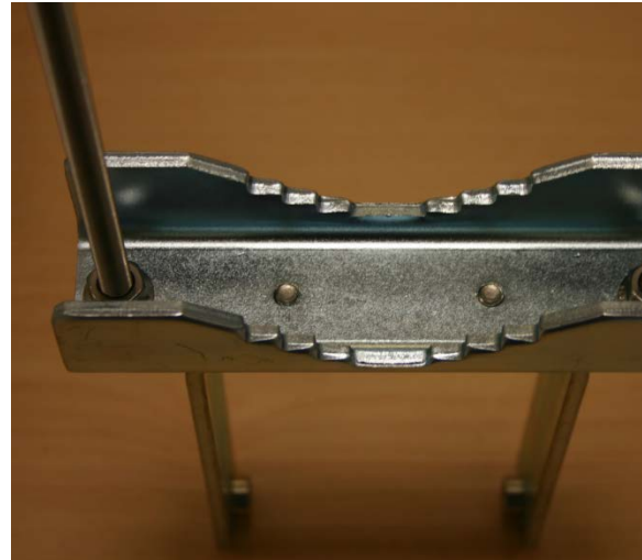
Figure 101 AP Antenna Lower Bracket Assembly
